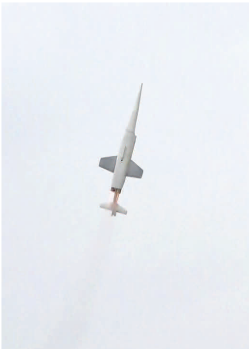
The X-3 Stiletto flew, but since it was designed for mini-B's, the two A's couldn't heave it high enough.
