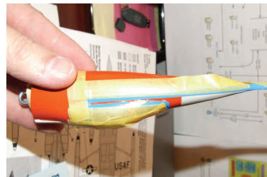
Figure 11 - Masking of the cockpit section
